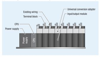
(3) If interference still occurs, leave the next slot open to secure a space for wiring.
