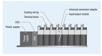
(3) If interference still occurs, leave the next slot open to secure a space for wiring.
