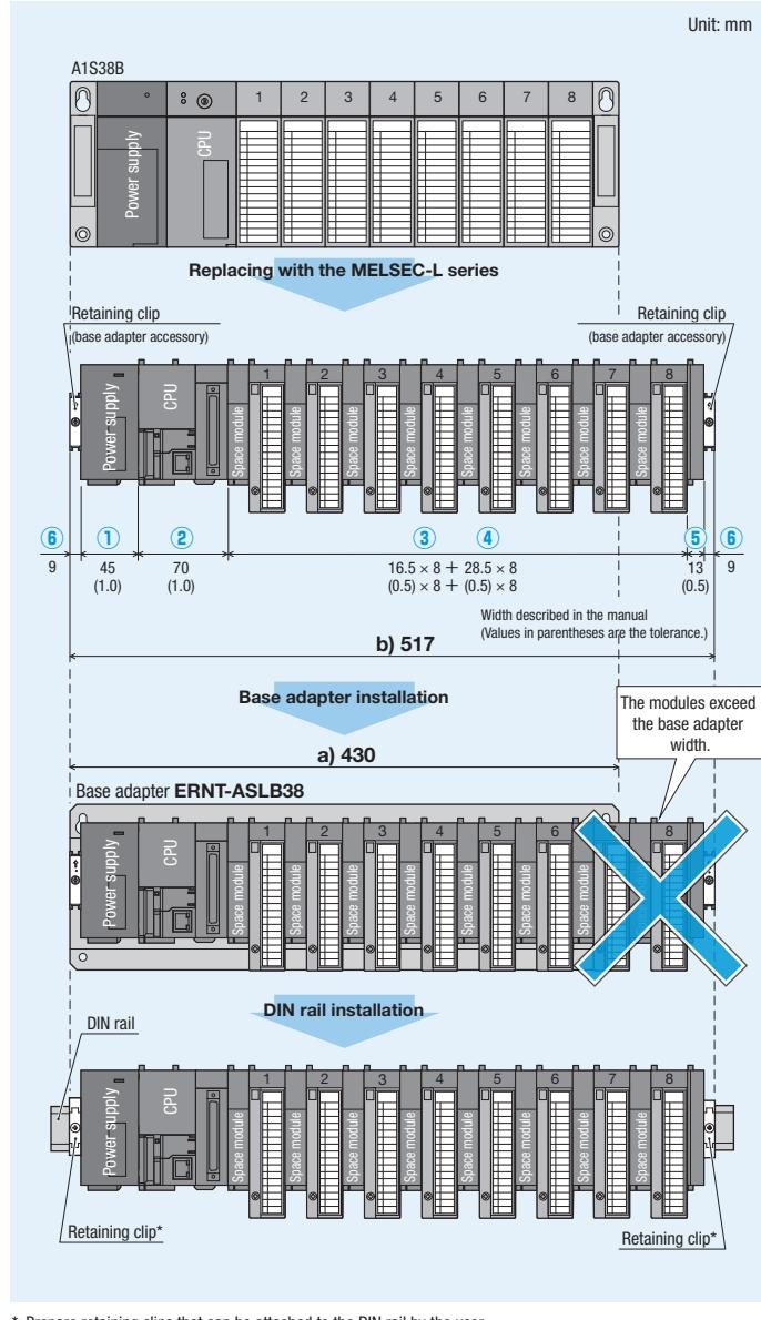
\*: Prepare retaining clips that can be attached to the DIN rail by the user.
