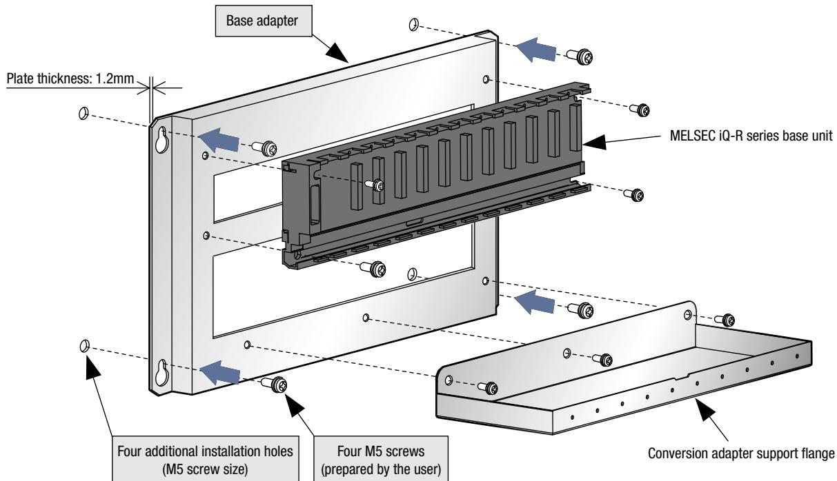
The base units (\*1 to \*3) can be installed to different types of base adapters. Select the optimum base adapter.
