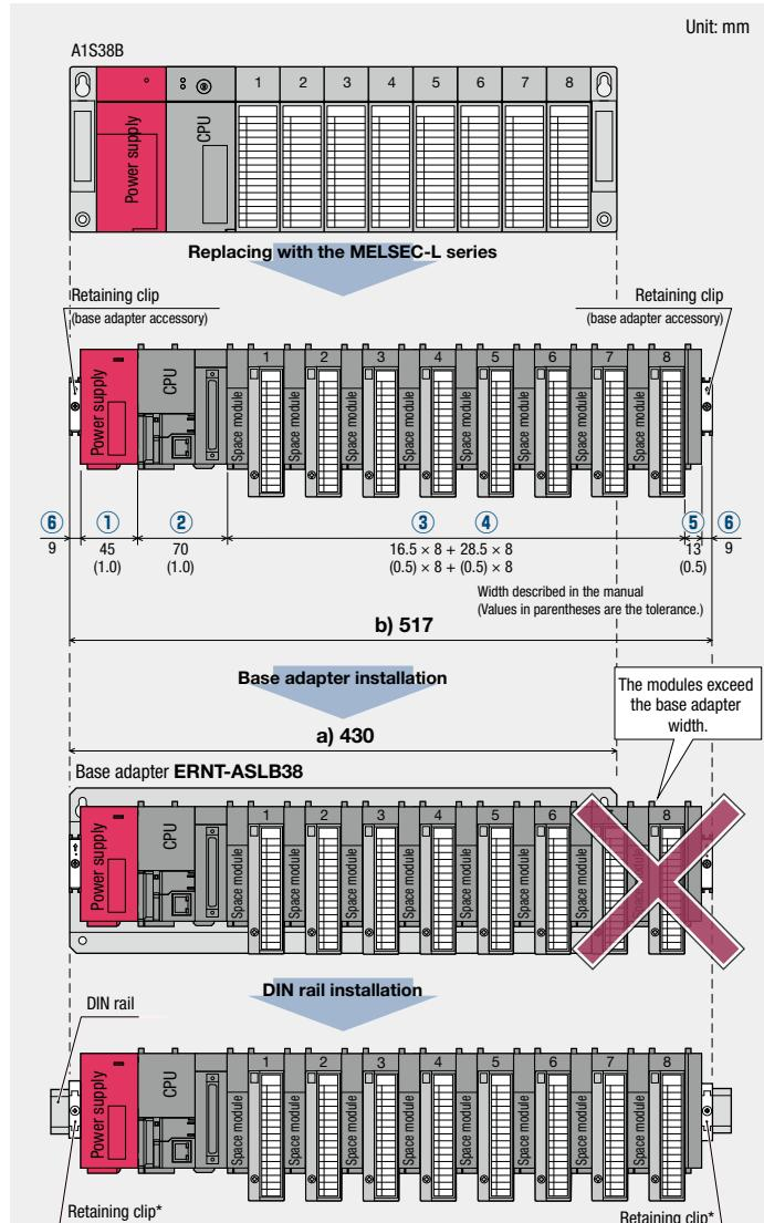
\*: Prepare retaining clips that can be attached to the DIN rail by the user.
